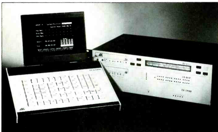
Audio Kinetics ES1.11 EBus synchroniser with mainly dedicated push buttons
