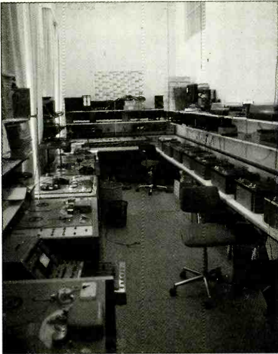
The duplicating room. A row of M10s to the left and A77s to the right are linked, via the mixer at the back, to all three studios
