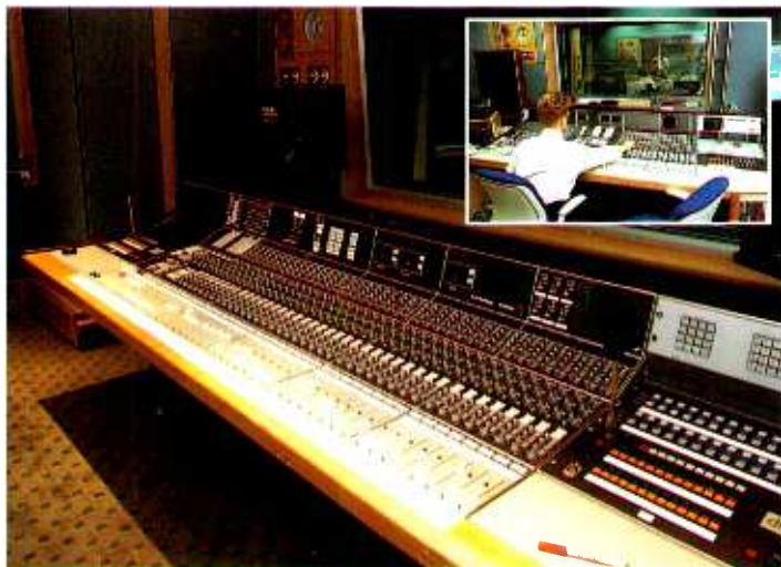
▲ 40 channel SL 5000 M Series console at BBC Radio 5 used for outside broadcasts, with (inset) the smaller 22 channel SL 5000 M Series
