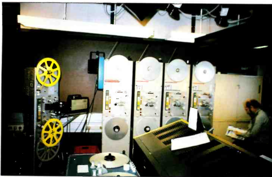
Machine room housing sep mags and telecine
