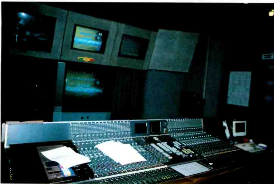
Main post-production room with Eclipse keypad and screen built into the mixing console
