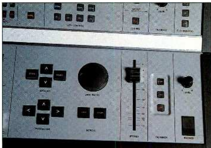
Data parameter and memory control section
