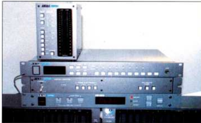
Top to Bottom: Akai's Digital Signal Patchbay; Sampling Frequency Converter and Digital Offset Editor for A-DAM
