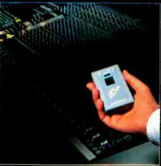
Wireless talkback system uses a PCM encoded infra-red handset
