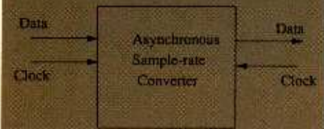
Fig.2b: Asynchronous sample-rate conversion. Ratio is sensed from user-supplied clocks and may be irrational, asynchronous and even time-varying!
