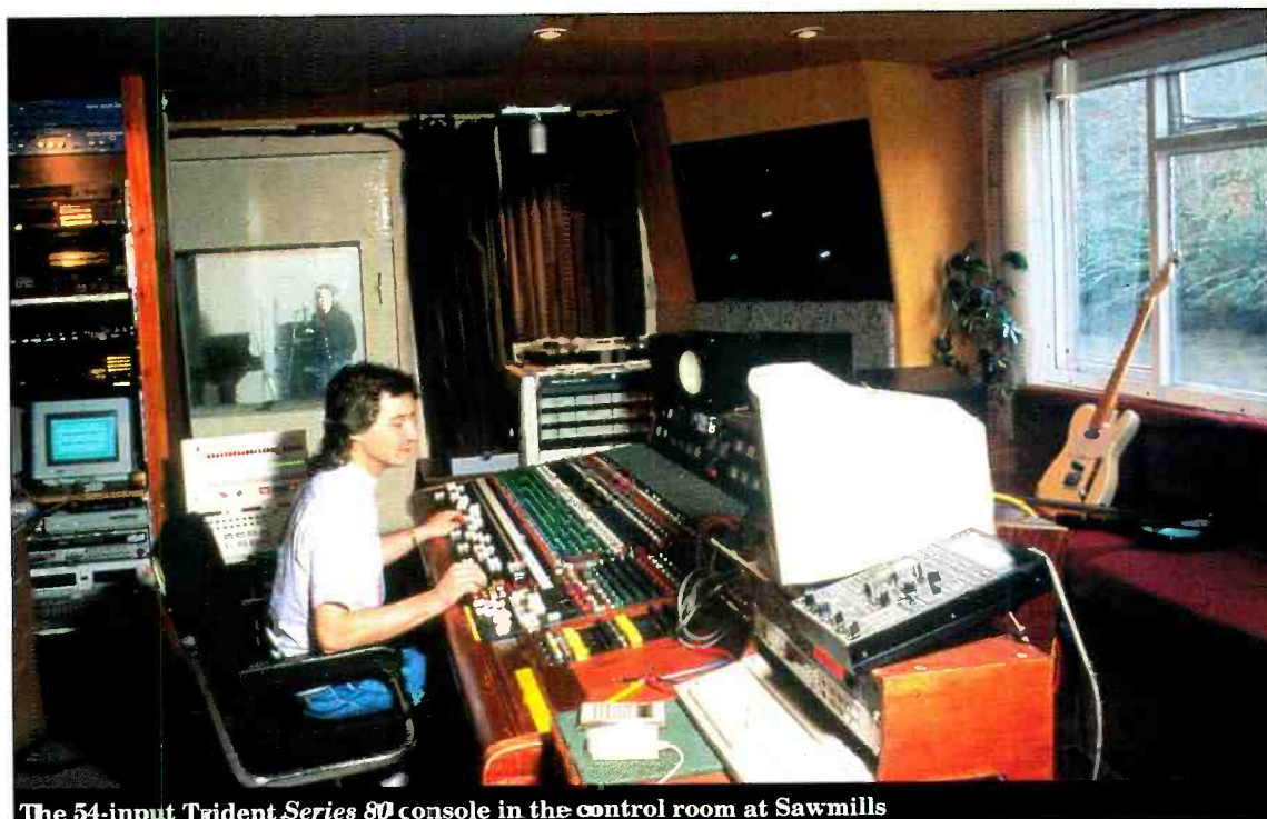
The 54-input Trident Series 80 console in the control room at Sawmills
