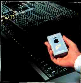
Wireless talkback system uses a PCM encoded infra-red handset
