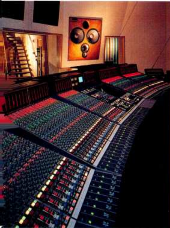
The Gallery's SL9000j backed by custom Boxer T5 monitors and custom ceramic diffusers
