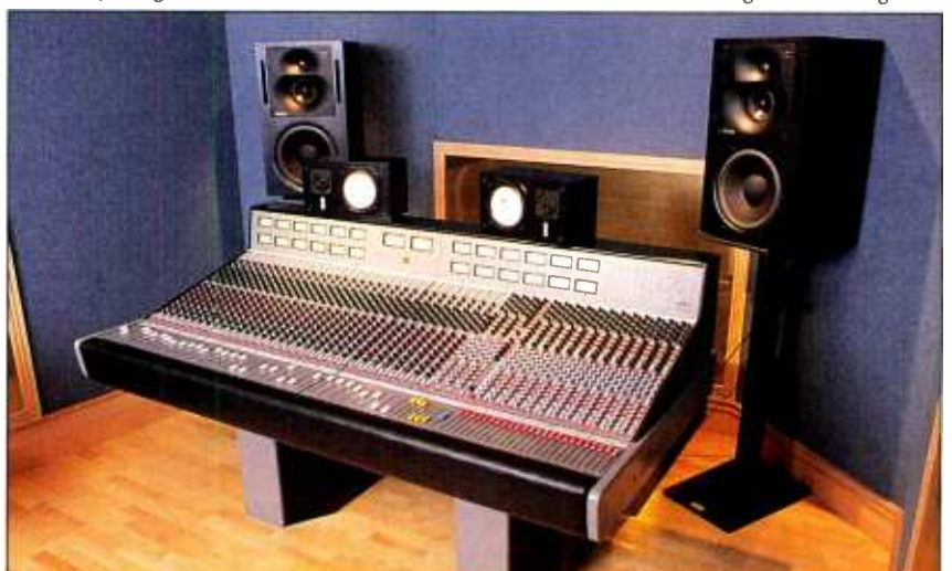
The console they agonised over: an MTA 980 was finally installed in Studio 2
