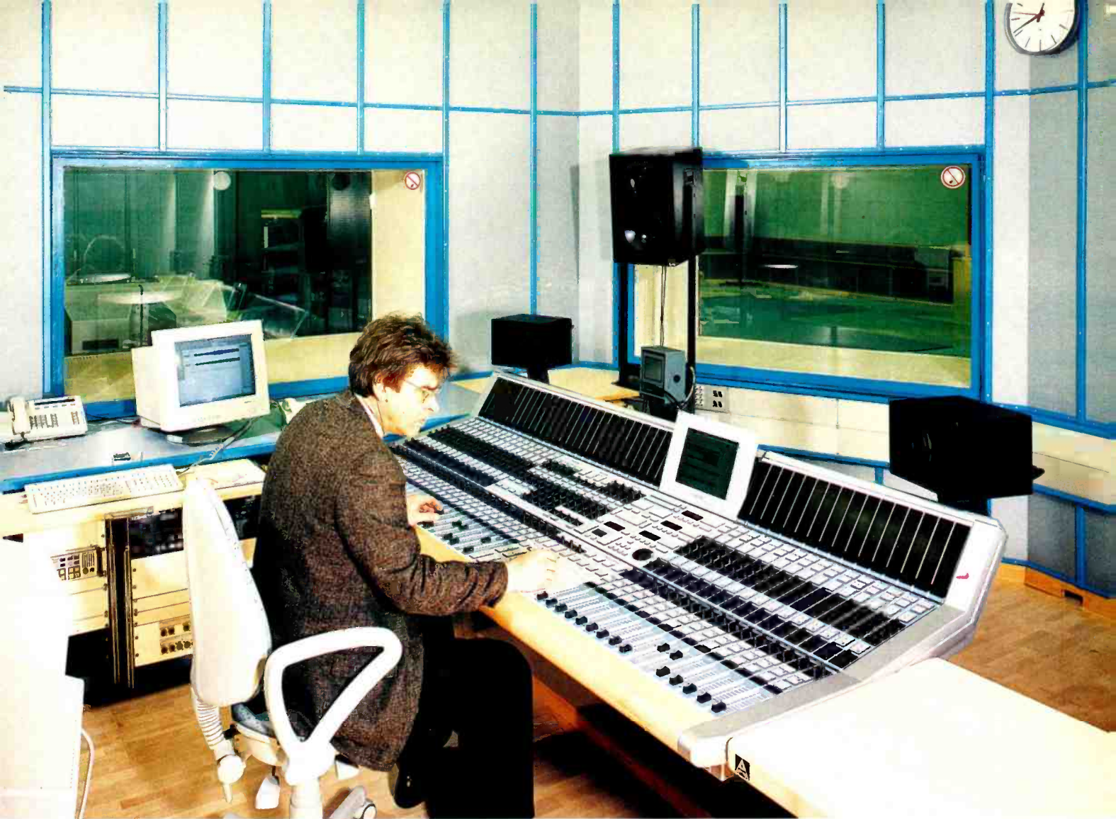
Studio Manager Hans Schmid at the Cantus console installed at Studio 10 Bayerischer Rundfunk (Bavarian Broadcasting) in Munich
