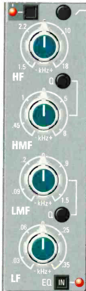
Above: REM 10 input module showing detail of routing arrangements—12 switches give access to Rembrandt's 24 buses. Note LED indicators. Right: EQ on both channel and monitor paths is identical, featuring four bands with switched Q on the two mid bands
