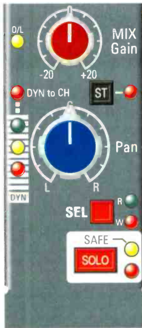
Above: Close-up of channel strip showing Virtual Dynamics LED indicators, channel automation mode selector switch, and monitor gain pot. Right: Aux sends featuring pre-post switching and access to 16 aux buses from eight sends
