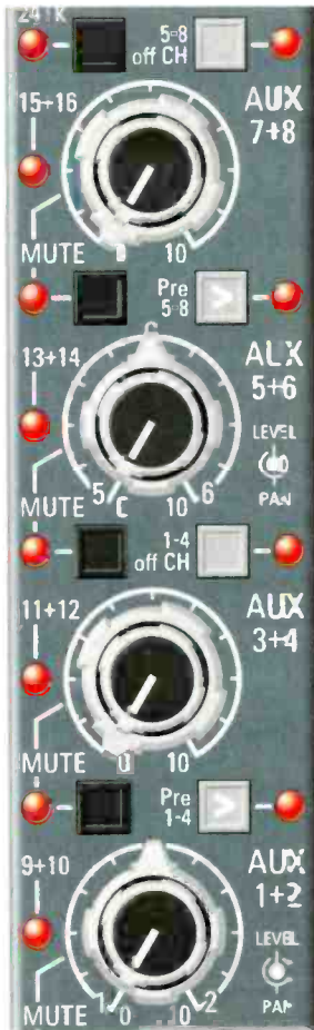
Above: Close-up of channel strip showing Virtual Dynamics LED indicators, channel automation mode selector switch, and monitor gain pot. Right: Aux sends featuring pre-post switching and access to 16 aux buses from eight sends
