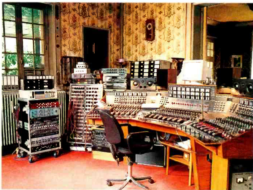
Mike Hedges' vintage EMI TG console at home in the control room
