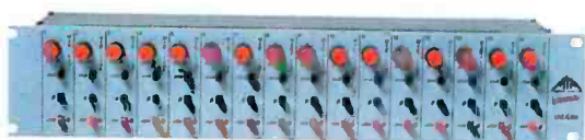
The mic-line module features phase reverse and individual 48V phantom power
