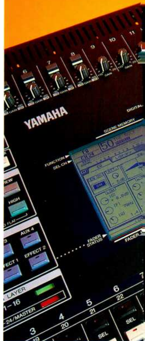
The 03D control surface has a total of 39 buttons for control functions plus two buttons associated with each of the 19 fader strips. The faders are 60mm throw motorised units.
