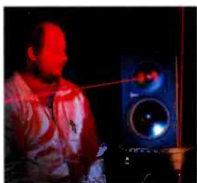
Mackie acoustic engineer David Bie uses scanning laser vibrometry to map HR824 tweeter dome vibrations.
