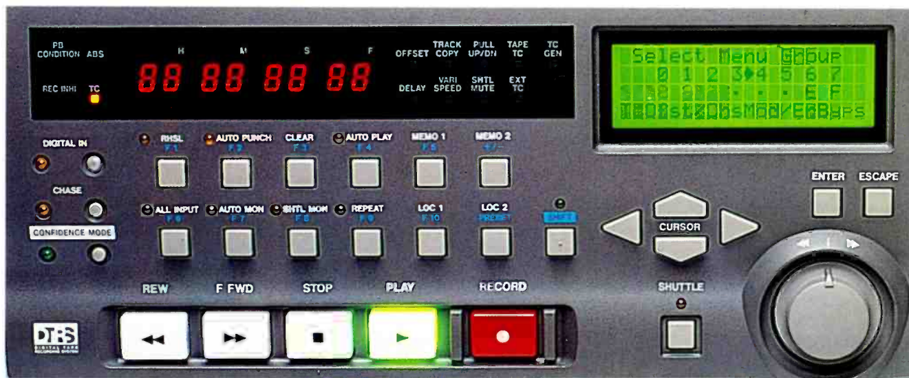
Close-up of the front panel showing transport and management controls including the new confidence monitoring facility
