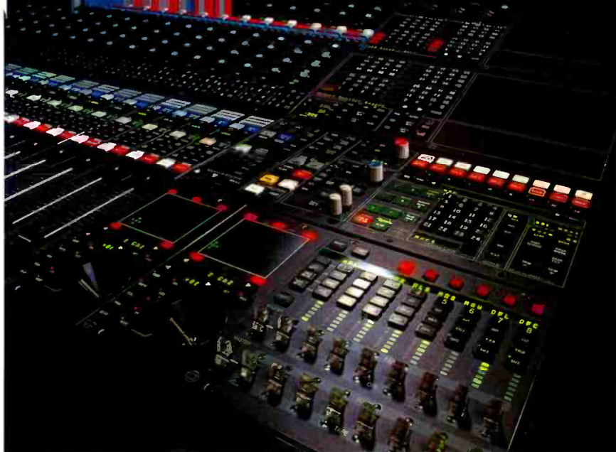
DFC Direct paddle switch panel and automated joystick controls
