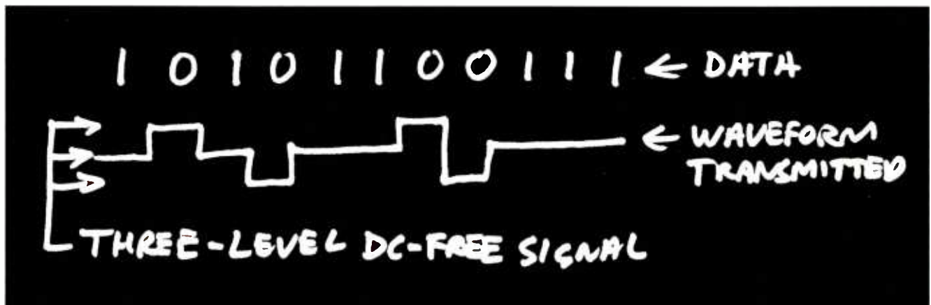
Fig.1: AMI coding eliminates DC from the data signal
