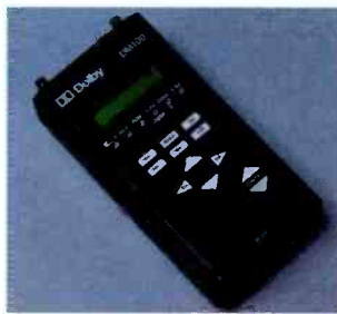
LCD displays Dolby Digital and Dolby E metadata information.
