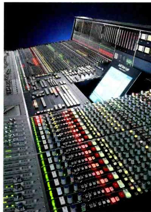
other consoles. Snapshots are recalled absolutely instantly, with no 'rippling' across the console. The immediacy of operation is the most important benefit to broadcast users. The new faders come with the useful 4-character display to show grouping and a slightly different feature set, such as backstop stereo PFL. The redesigned display is far less complicated than the sister consoles' displays, as befits the broadcast situation.
