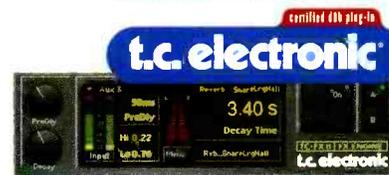
**TC Electronic Reverb** (bundled with the D8B UFX card) provides Reverb 1 and Reverb 2 algorithms from the renowned TC Electronic M2000 Studio Effects Processor.
