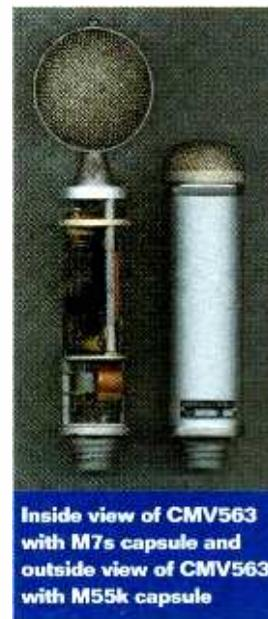
Inside view of CMV563 with M7s capsule and outside view of CMV563 with M55k capsule
