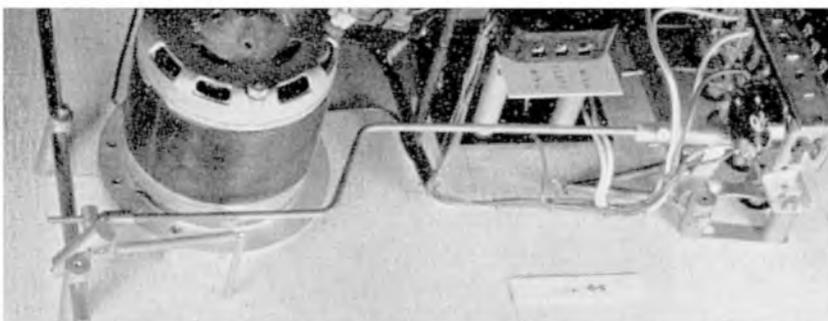
**Fig. 2:** The brake connection, noted above, can be followed in more detail here, with the tension spring immediately below it. To the left of the spooling motor is the link for that particular brake. Adjustment is effected by slackening off the grub screw and altering the angle of the lever on the shaft.
