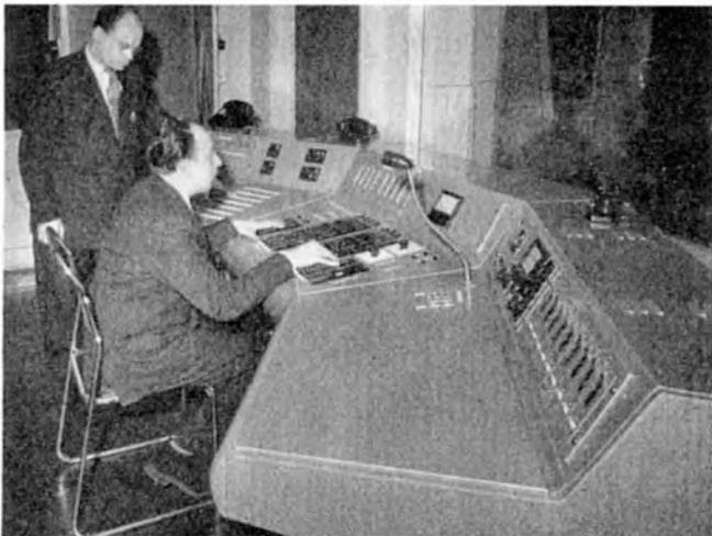
Professional mixers may have a dozen or more channels as shown in this photograph of the control console at a Philips recording studio.
