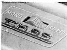
Turn this speed change control, press the button marked '1 1/2' and you get six hours playing time per tape.
