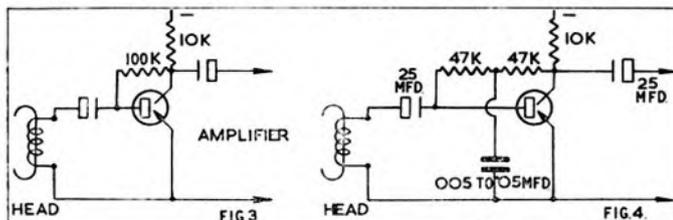
obtain the full gain of the transistor just where it is wanted. It should be pointed out that full gain is also available at very low frequencies where the impedance of the head has fallen to a low value so that the feedback is again very low. Fig. 4 shows the modified circuit.
