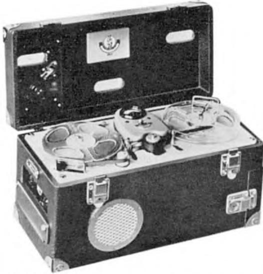
● The **L2/TA** is the latest version of the famous E.M.I. L2 professional battery portable. It is fully transistorised, and operates at  $7\frac{1}{2}$  i/s. Full details will be given next month.
