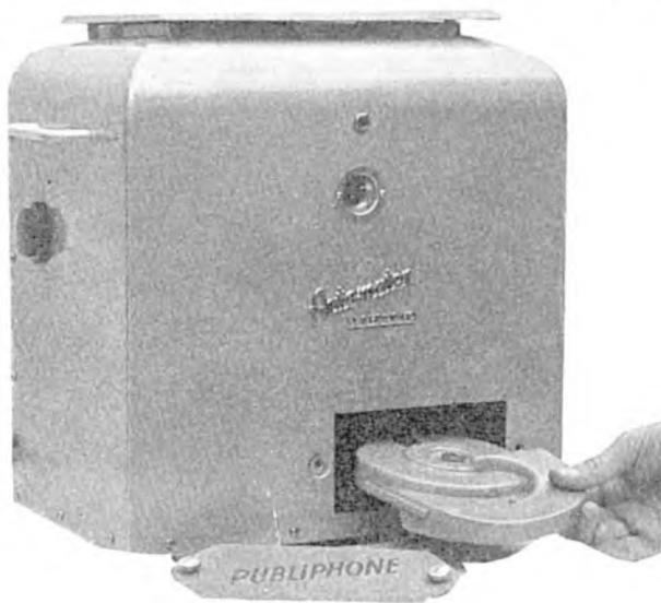
Inserting the tape cassette into Publiphone and Informatron machines takes a matter of seconds, so that the recording may be changed easily.
