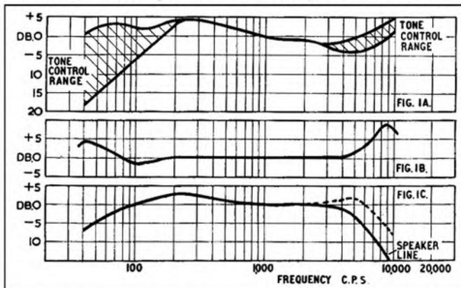
of note by any prospective user, is that the maximum bass is obtained with that control at the counter-clockwise end, whereas maximum top is obtained with the "top" control at the clockwise end of its travel. There is a convention, though I am not sure that it has official backing, that the maximum output of whatever is controlled should be obtained with the control at its
