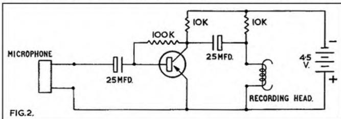
are trying to record. It will be seen that the direction of this current through the head is important, as it *must* produce a field across the recording head gap which cancels the saturating field, and allows both the positive and negative going half cycles of the signal to produce equal changes in the magnetisation of the tape oxide.
