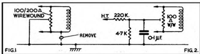
Figs. 1 and 2. Circuits illustrating the use of a humdinger potentiometer. The values of components may vary from those shown.
