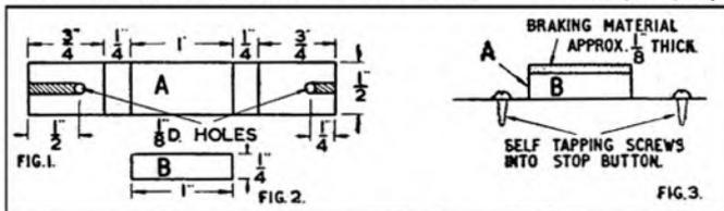
The brake is made from a small piece of tinplate attached to the underside of the Stop button. Braking action is obtained by friction between the brake material and the ridges on the flywheel.
