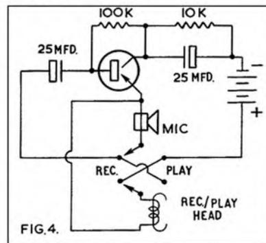
Fig. 4. Shows a method of using a double-pole, double-throw switch to change over the transducer and the Record/Replay head for recording or playing back. This diagram is included for experimenters who are able to assemble more complicated arrangements helped by the circuit above.
