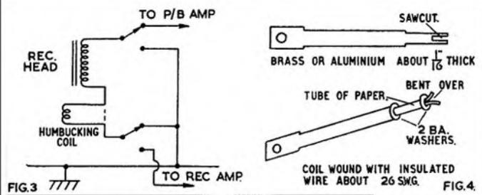
Fig. 3. (Left). Typical head switching circuit, showing the use of a humbucking coil. Fig. 4. (Right). A thin dural mount as shown allows the coil to be tried in different positions for best effect.
