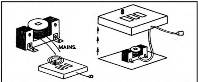
shown. Thin plastic was used for the top of the box, but no doubt Perspex or even Formica would do equally well.
