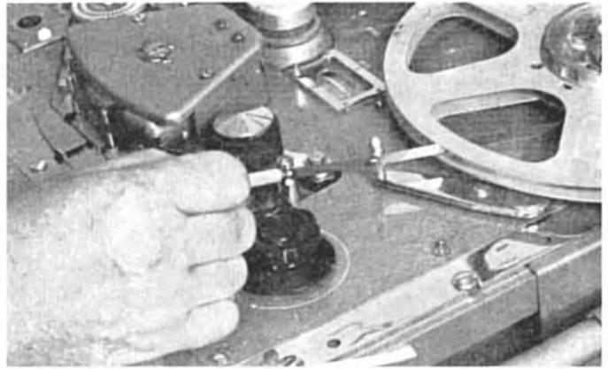
*Accurate marking is essential, and when the replay head is inaccessible you should find a fixed offset point, e.g. a tape guide as shown. (BBC Photo).*
