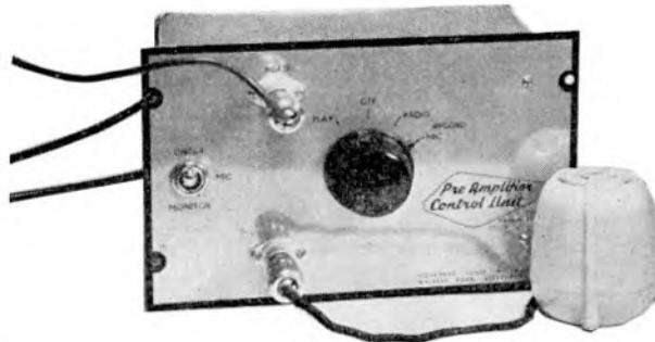
The switching facilities for record and replay with the transistor amplifier, described last month, are incorporated in the Author's Gramdeck amplifier.
