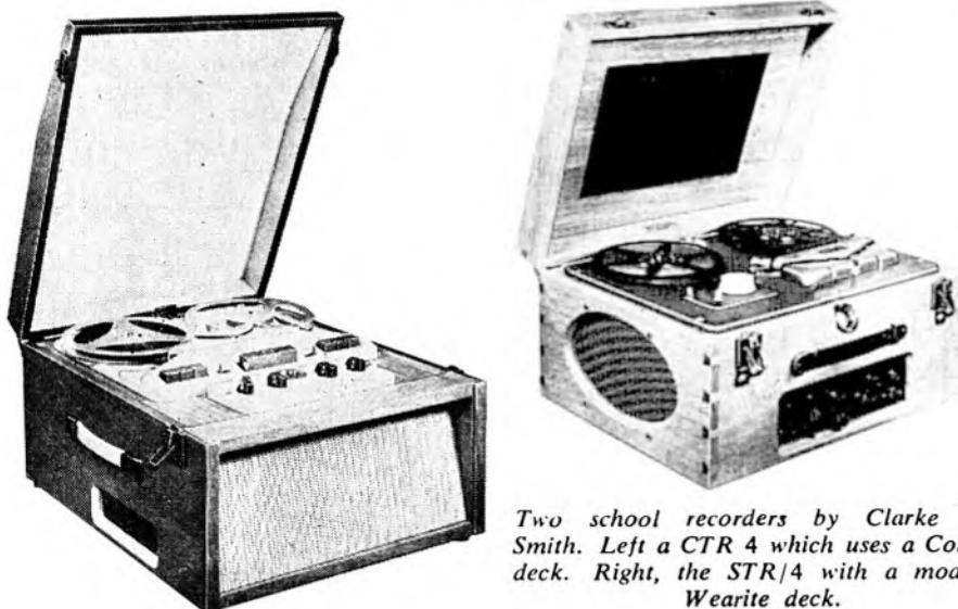
Two school recorders by Clarke and Smith. Left a CTR 4 which uses a Collaro deck. Right, the STR/4 with a modified Wearite deck.
