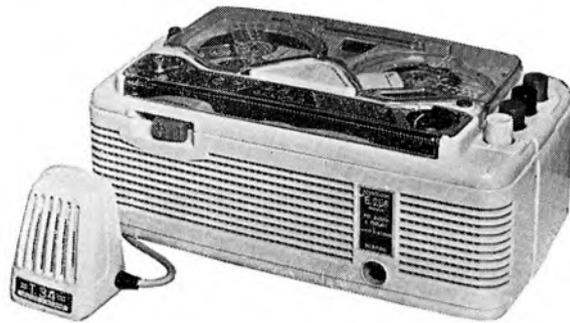
High-quality reproduction at  $1\frac{3}{4}$ " per second from extra high flux elliptical speaker. B.S.S. tracking. Simple push-button control. Accurate place indicator. Dimensions  $10" \times 5\frac{1}{2}" \times 4"$ . Weight only  $6\frac{1}{2}$  lbs. Isolated chassis.
