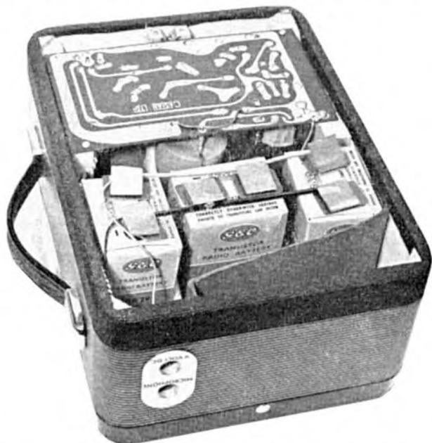
Rear view, with back removed, showing the printed board, batteries, and microphone storage compartment.
