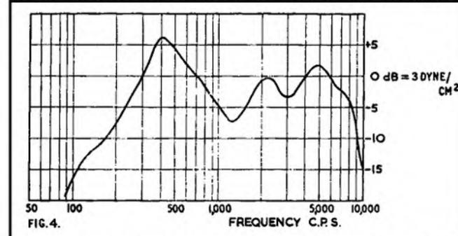
pushed up to 400 c/s by the small internal volume of the recorder case. The resultant peak is undamped and gives a slightly "boxy" quality to the radiated sound.
