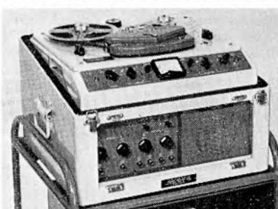
seen as well as heard! The latest stereo recorder from *Vortexion* is the CBL, with mixing of inputs, stacked heads and over 6 watts total output. Meter monitoring of bias and signal, and facilities for recording from track to track with additional signals, are features of note. Entirely separate low impedance micro-
