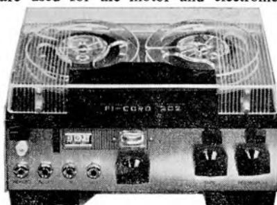
cells being loaded in interchangeable cassettes. Expected battery life is 30 hours for the motor (at 3½ i/s) and 60 for the circuit. A line output provides a signal of one volt maximum, while a built-in speaker may be driven at 180 mW. Fast forward and rewind, a VU meter and response flat to 12 Kc/s at 7½ i/s make this a versatile high quality recorder. Price is 66 guineas.
