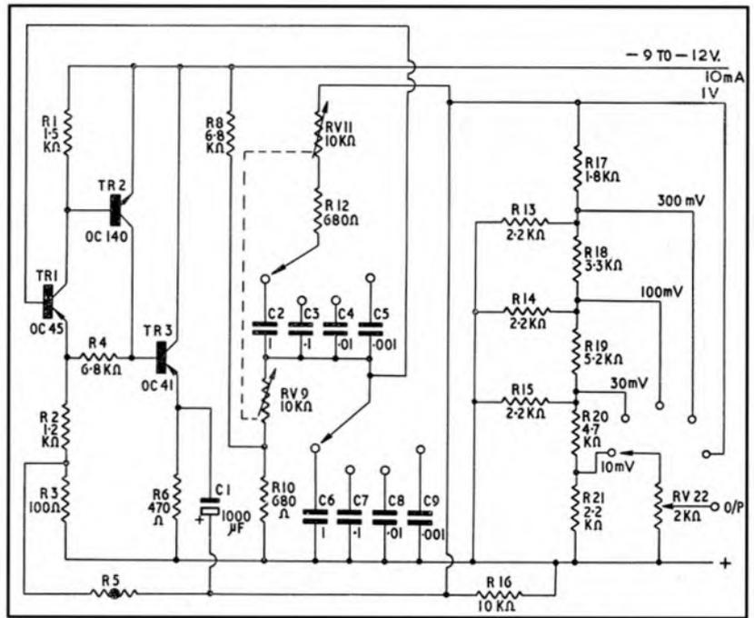
IN the November 1962 issue of *The Tape Recorder* I described an A.C. millivoltmeter that I have been using for several years. In order to use such an instrument to its fullest effect as a piece of test gear, particularly in respect of tape recorders, a second unit is needed. This second unit is an audio oscillator, again the one I have been using for a considerable time was home made.
