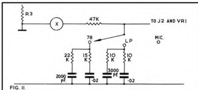
Fig. 11. A suggested lossier equalising circuit.
