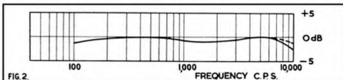
level frequency response or standard playback level, the bias is varied to see if matters can be improved and the bias change noted and mentioned in the review. In this sample the bias proved to be optimum, and the playback level was only 1 dB below standard Fig. 1.
