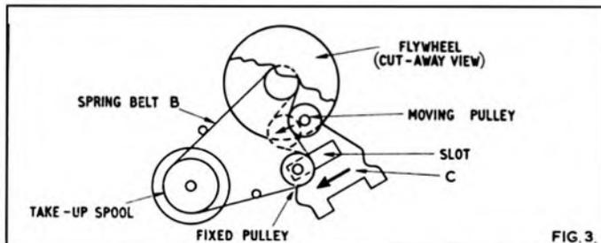
spool) depends on the driving axle at each end of the motor engaging its appropriate rubber ring beneath the spool carriers. These axles should be equidistant from the rubbers, and a little judicious bending of the brackets to which the springs are attached may be needed. But note that there is an axial play of 0.08 in. of the Rewind motor, which is quite normal.
