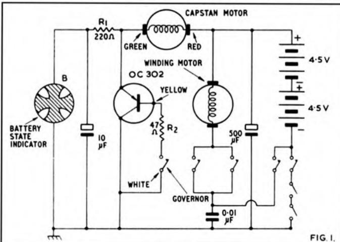
in **fig. 1**. Note the two 4.5 volt batteries in series, supplying the motors with 9 volts. The amplifier has a separate power supply, also 9 volts.
