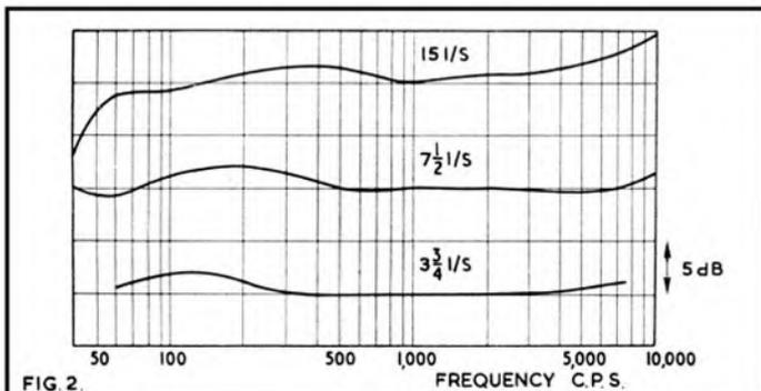
tape level was recorded at a scale reading of 2 on the record level meter and peak recording level (plus 12 dB on test tape level) was recorded at a meter reading of 6. At this reading, waveform distortion was small but increased appreciably when the meter reading was raised to 8.
