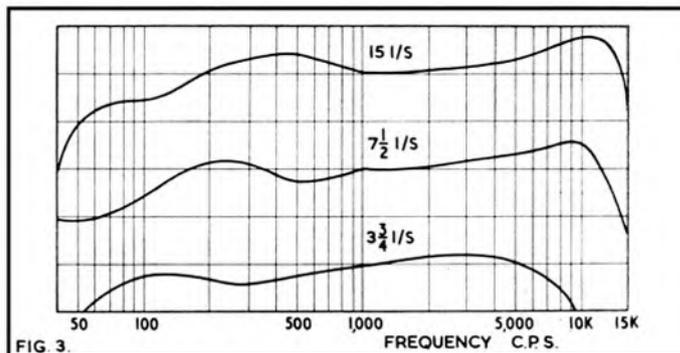
at  $3\frac{3}{4}$  i/s confirms that the bias was indeed about right for the tape speeds provided by this deck—a little high for  $3\frac{3}{4}$  i/s—a little low for 15 i/s—and just right for  $7\frac{1}{2}$  i/s. For a lower speed deck 40 volts bias would probably be all right. The response on the lower track was next tested and found to be almost identical to that of the upper track.
