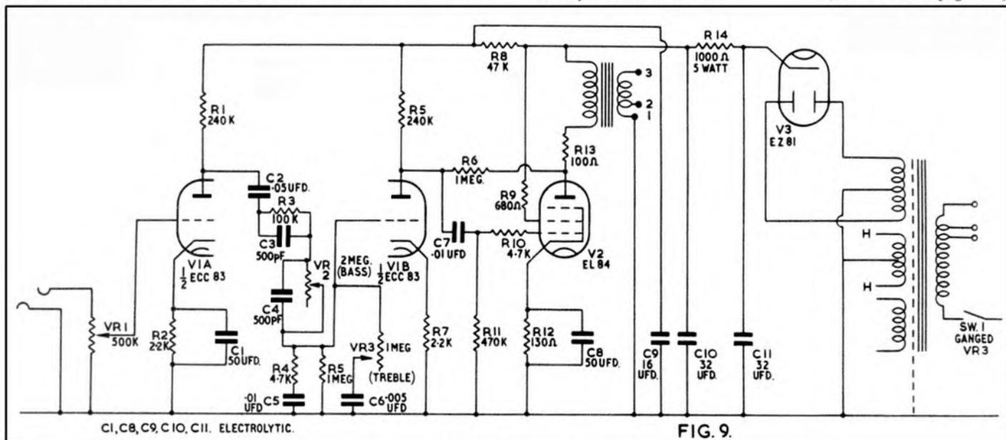
Fig. 9: Circuit diagram of the W.B.U. power amplifier suitable for use with the TW/PA4.
