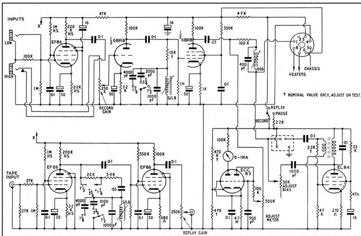
Fig. 1A: Circuit diagram and component values for use with the Planet U1 tape deck. Since passing this for press the author has sent in the following alterations: 220 Kohm resistor should be placed between the anode of the first half of the 6BRB valve and 0.1μf capacitor. The 30K bias adjuster open side should be taken to chassis.
