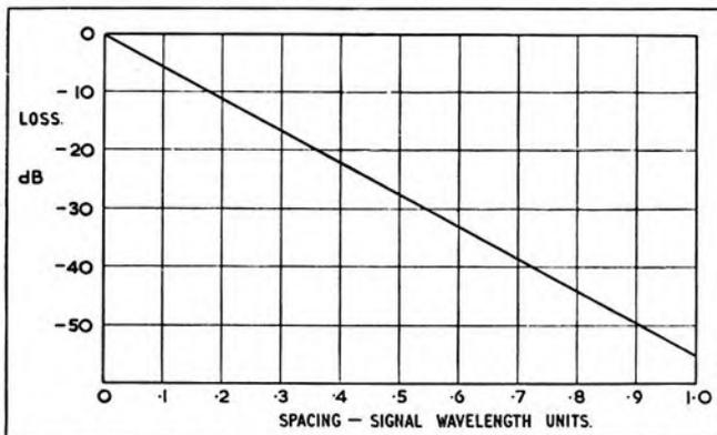
Fig. 2: Effect of Head-Tape separation. The horizontal scale can be read directly (full-scale = 1 thousandth of an inch) for a signal wavelength of 1 thou', e.g. 7.5 Kc/s at  $7\frac{1}{2}$  i/s, 3.75 Kc/s at  $3\frac{1}{2}$  i/s, 1.875 Kc/s at  $1\frac{1}{2}$  i/s, etc.; or with full-scale of half this for twice these frequencies and similarly for other wavelengths in inverse proportion.
