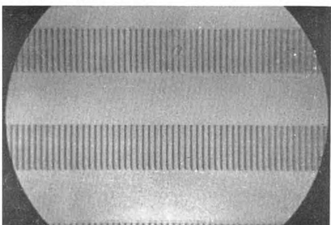
**Fig. 5:** Tape blemish, 1963 style, but actually a small nodule on 1958 thin-based tape. Actual magnification x 18, but would represent present conditions at magnifications of 100-200. Actual size of blemish about 5 thou' diameter x 1 thou' high, about ten times the average modern pimple.
