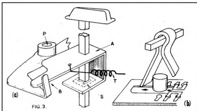
the slider and the mounting bar. The resistor is an arc of composition track on the reverse of the component as shown, and the slider is an arm which has a circular base. This base is formed to sit in the circular aperture so that two lips ride on the rim. If the control has been adjusted clumsily, with a screw-driver that does not fit the central slot, the contact between lips and rim loses efficiency.
