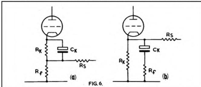
**Fig. 6.** Methods of negative feedback injection, alternative to that in **fig. 7**. (a) may be noisier than (b) because in it DC flows through  $R_f$
