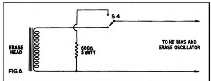
In my recorder, the leads from the erase head are soldered to the upper tag-strip on the output transformer. This is the best point at which to make the switch connections.
