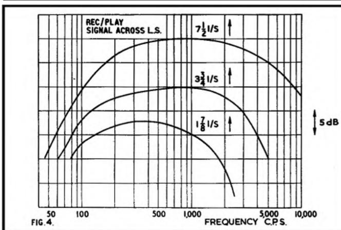
A signal 13 dB above test-tape level was recorded without distortion with the magic-eye beams just closed, and hum and noise across the LS voice-coil was 36 dB below test-tape level, so that the total dynamic range or signal/noise ratio was 48 dB. Recorded noise was only 2 dB above that of bulk-erased tape. The low hum level is partly due to the sharp fall in low note response below 200 c/s.
