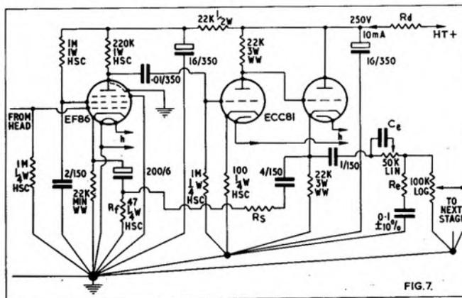
**Fig. 7.** Low-noise pre-amplifier block followed by basic series playback equaliser. Heater pairs (h) connect to 6V DC supply.  $R_s = 22-100\text{ K}$ , 1W HSC, according to gain requirements. Adjust  $R_d$  to give 250V DC where shown.  $C_e$  is approx.  $\cdot 001\text{ mfd}$  for 15 i/s or  $\cdot 002$  for 7½ i/s. 50K pot gives HF compensation for head losses.  $R_e = 300\text{ ohm} \pm 10\%$  for 7½ i/s, gives LF compensation with  $0\cdot 1\text{ mfd}$
