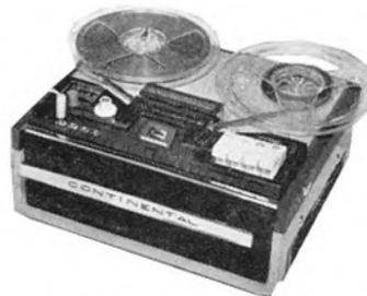
on the belt which was rough in texture and irregular in cross section, so that the ratio between motor speed and flywheel-capstan speed depended on how the belt happened to lie on either pulley at any instant.
