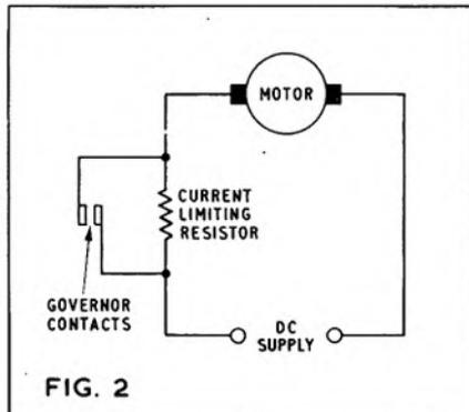
is too low for correct operation of the tape deck. This condition may not be satisfied on a new battery should the value of the resistor be too low. A small degree of speed adjustment is possible by the contact adjusting screw, but as this is accurately set at the factory it should not normally be re-adjusted by the user.
