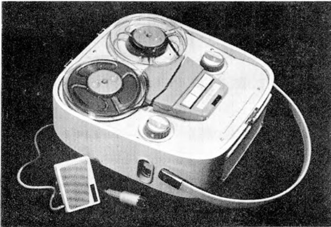
access to microphone and batteries. This was held in place by a screw which could be engaged easily with a coin. It was found difficult to replace the lid satisfactorily once the microphone had been extracted and replaced, this being another case of the microphone and cable being just a little too big.
