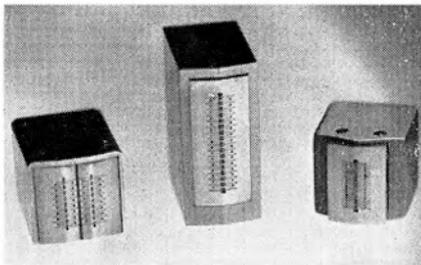
UP to 32 tracks on 1in. tape are possible with heads in the range lately announced by *Electro-Mechanical Systems Ltd.* Ferrite cores are employed in all record/replay heads, with effective gap widths of 1 micron and above. Bases of two thicknesses are available for special applications requiring the interlace of two adjacent heads. EMS heads are available in all standard configurations and also to *SBAC* and *IRIG* standards.
