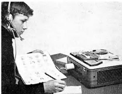
BRITIMPEX are now handling a 'Mini-Lab' Language Laboratory based on the *Luxor MP283* mono tape recorder. A variety of accessories are available for the system, including six-way distribution boxes through which pupils may monitor with headphones the language course from a single recorder. Up to five of these boxes may be fed from one recorder, allowing 30 pupils to participate. The *MP283* is being marketed at £62 9s. 6d., excluding earphones, microphones and amplifier.
