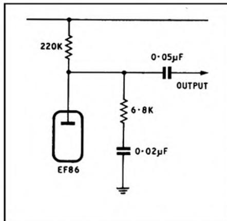
The circuit illustrated here may be added to each output to provide 140µs equalization. This will give a response roughly in accordance with the *DIN/CCIR* standard for 3 1/3 i/s operation, though the mid-frequency gain of the circuit will be correspondingly reduced by about 25dB. As modified, the circuit should only be used when the input impedance
