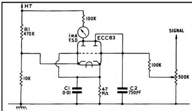
The circuit is straightforward. The 470K resistor R1 could be altered to give exact balance, and if you want a better delay characteristic (this is a peak-reading type) increase C1 to 0.015 or 0.02mF. The capacitor C2 is important, being 750 pF and preferably a good disc ceramic, as this one performs the function of by-passing the bias from the detector.
