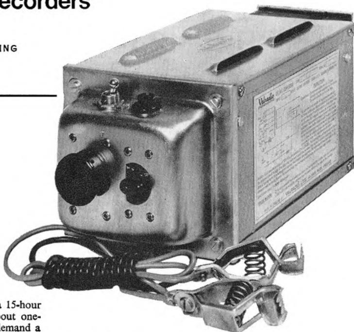
**T**O charge a nickel-cadmium cell fully, something like a 15-hour charging rate is required at a charging current of about one-tenth the cell capacity. Thus, a cell of 200 mA/h would demand a charging current of about 20mA for 15 hours. After this time, assuming a cell in good condition, full cell capacity will be restored.
