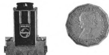
Fig. 4 (above): Philips video head shown life-size.
