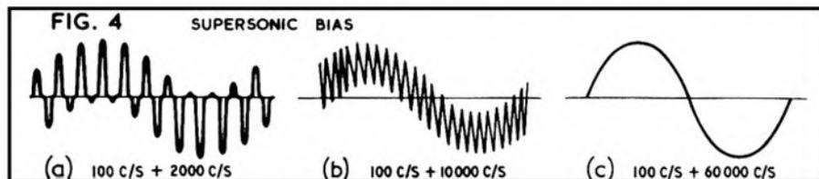
and 2 Kc/s are superimposed in a record head. We can see that the result is a high-frequency recording whose average amplitude varies at the lower frequency. There is no low-frequency distortion because the magnetic field is alternating too rapidly for the low frequency transfer-characteristic to apply.
