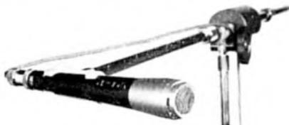
Frequency response (to -2dB points) is from 70 c/s to 16 Kc/s, and sensitivity (30-50 ohms impedance) is 88dB below 1V/dyne/cm<sup>2</sup>. Polar response is omni-directional, partially suppressed at the rear. The low-impedance *CPDL* retails at £15, while the medium and high impedance *CPDM* and *CPDH* are £16. A non-switched *CPDL*, is available at £14. Manufacturer: Reslosound Ltd., 24 Upper Brook Street, London, W.1.
