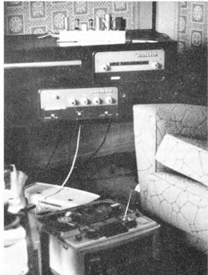
FIG. 5 FISHER DECODER COUPLED TO A HEATHKIT FM-4U TUNER.
