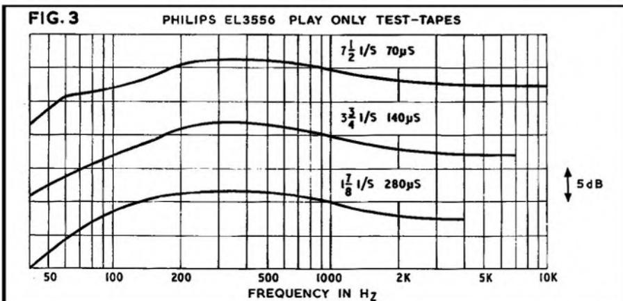
THE Philips EL3556 is in the higher price bracket for a mono  $\frac{1}{4}$ -track recorder, but it offers a very wide range of tape speeds, a higher than usual power output and wide range bass and treble tone controls to make the best possible use of the well equalised responses on internal or external loudspeakers.
