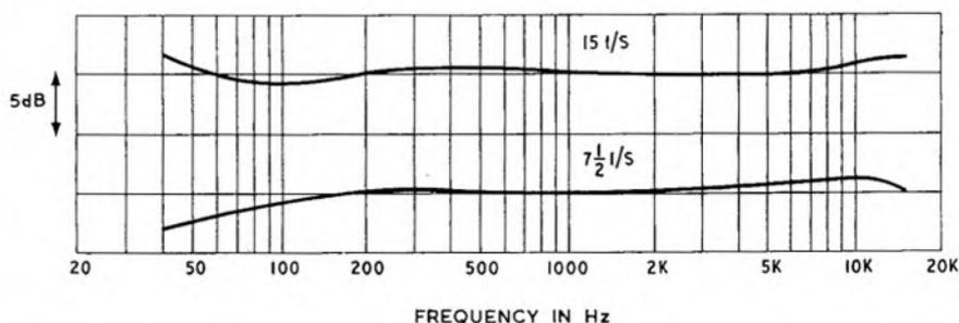
FIG. 4 REVOX 736/HS ACOUSTIC RESPONSE
