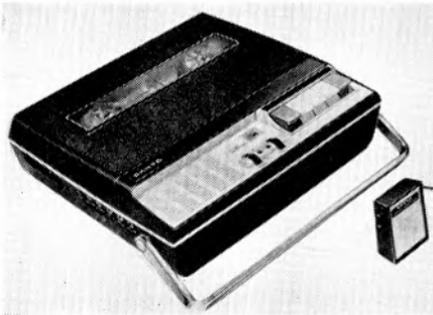
Quarter-track stereo recording facilities are included on the *MR.151*, which has speeds of  $3\frac{3}{4}$ ,  $1\frac{1}{2}$  and  $\frac{1}{8}$  i/s and takes 5in. spools. Output power is quoted as 0.9W per channel through internal side-facing speakers. Pause control and twin VU-meters are incorporated. This model operates from six U2-size cells or mains and has a 35dB signal-to-noise ratio. Price has yet to be decided.
