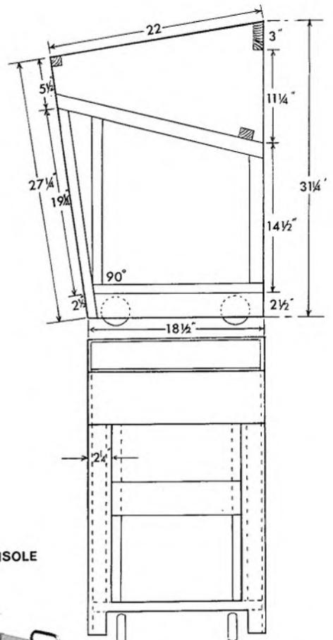
FIG. 7 CONSTRUCTION OF CONSOLE
