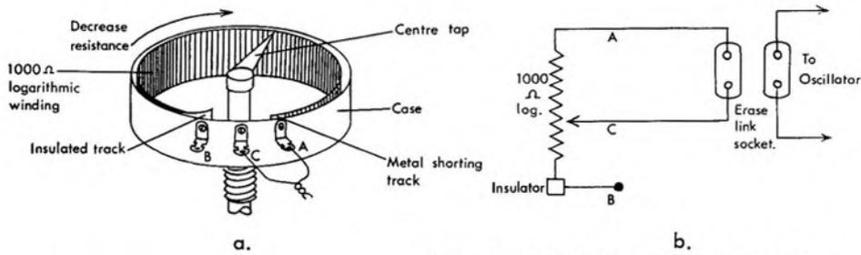
FIG. 1 DETAILS OF INTERJECTION CONTROL
