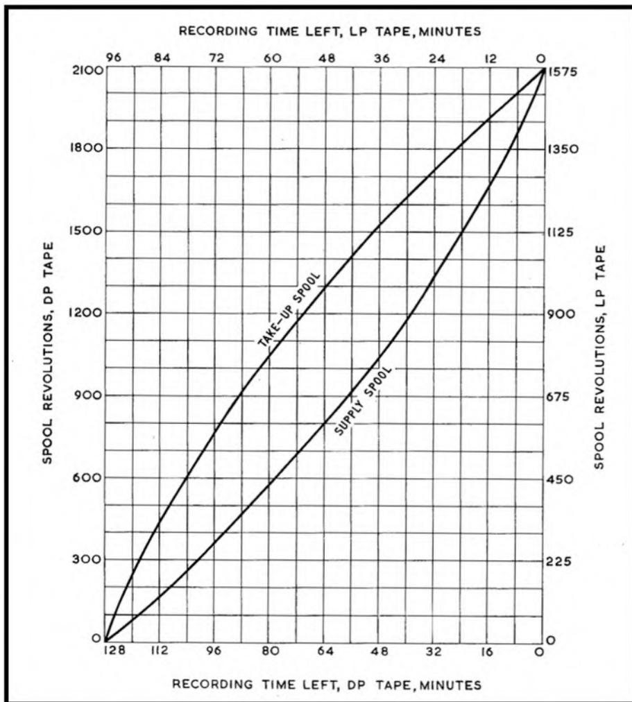
revolutions should have a total count of about 700 for 2400ft. of DP tape on a 7in. reel.
