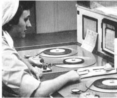
A sample of domestic tape from each block is inspected to ensure consistent quality.
