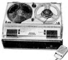
½ Track Mono recorder. Tape Speed 3½ i.p.s., takes up to 5½" reels. Frequency response 60 to 12,000 c.p.s. Manual and Automatic recording level control. Dimensions 13½" x 10½" x 6½". Weight 22lb.
