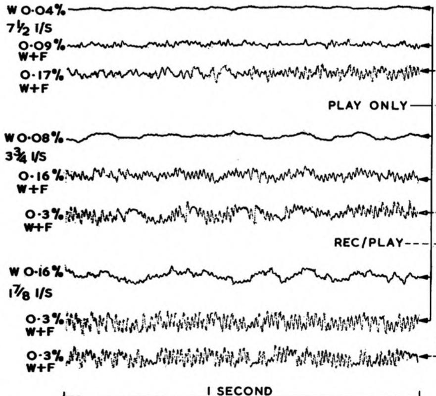
wind or rewind. Long term tape speeds were measured by strobe tape and constant frequency tapes and found to be within  $\pm 2\%$  limits over a 5 $\frac{1}{2}$ in. reel at all speeds.
