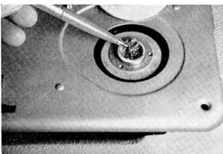
Result of loose drum on the foregoing deck. The motor spindle wears away the softer metal of the turntable. Eventually, the assembly seizes and the motor may be ruined.
