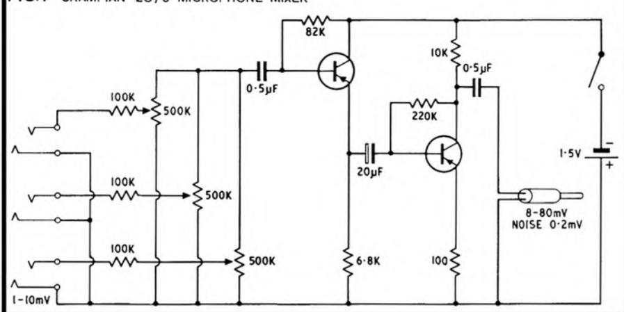
potentiometer so that the signal is earthed when the control is at zero, and most of the microphone signal is fed to the input of the transistor amplifier when the control is at maximum. The input impedance of the emitter follower input stage is about 50 K so that the mixer loss is about 3:1 or 10 dB.
