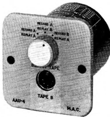
fed from a 100 k source into a 200 k load between any terminated input and output. Crosstalk was also negligibly low, being not greater than -40 dB at 10 kHz with 200 k loads, between any pair of connections. Care should be taken to keep external leads as short as possible. The screened leads are retained only by a rubber grommet and liable to some strain on the soldered joints.
