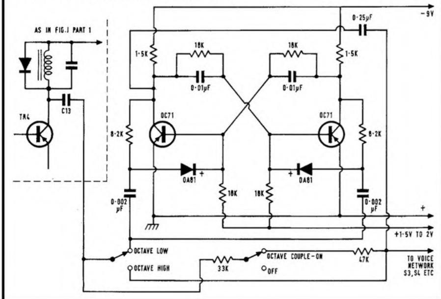
FIG. 8 DIVIDER POWER SUPPLY
