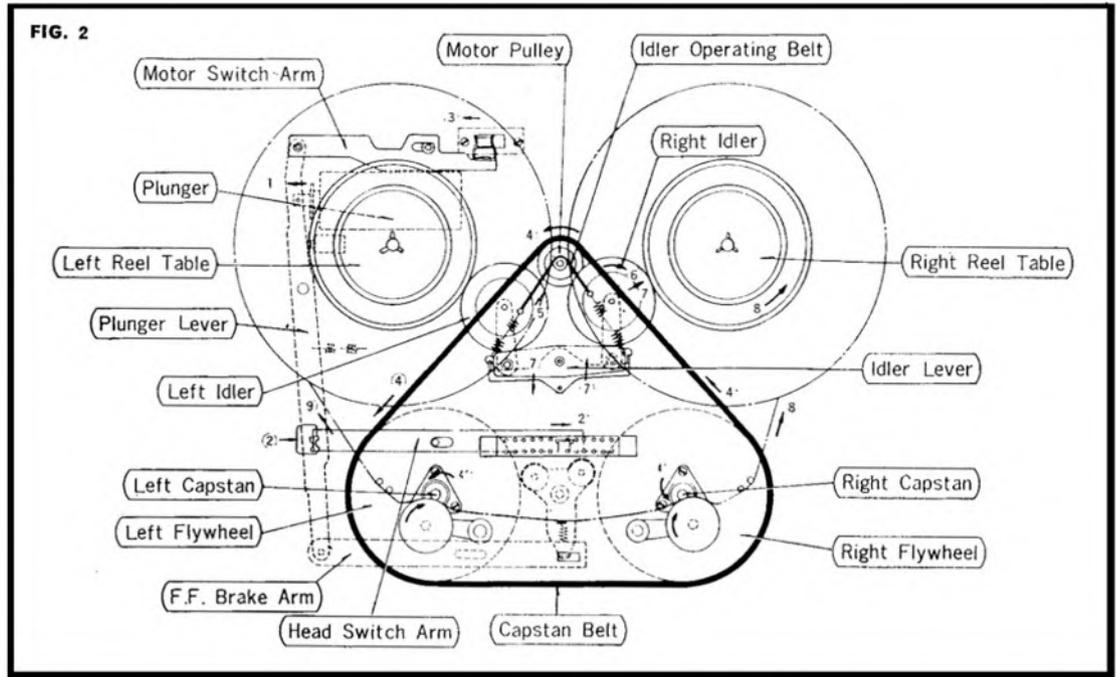
that of the previous one. From flywheel A back to the motor there is hardly any tension at all; there is no load on this part, in fact the motor is 'paying out' so one would expect this part to be slack. In practice, of course, the belt is slightly smaller than its path, so it needs to be stretched when fitted, hence no part is actually slack otherwise no grip would be exercised on the flywheel surfaces.
